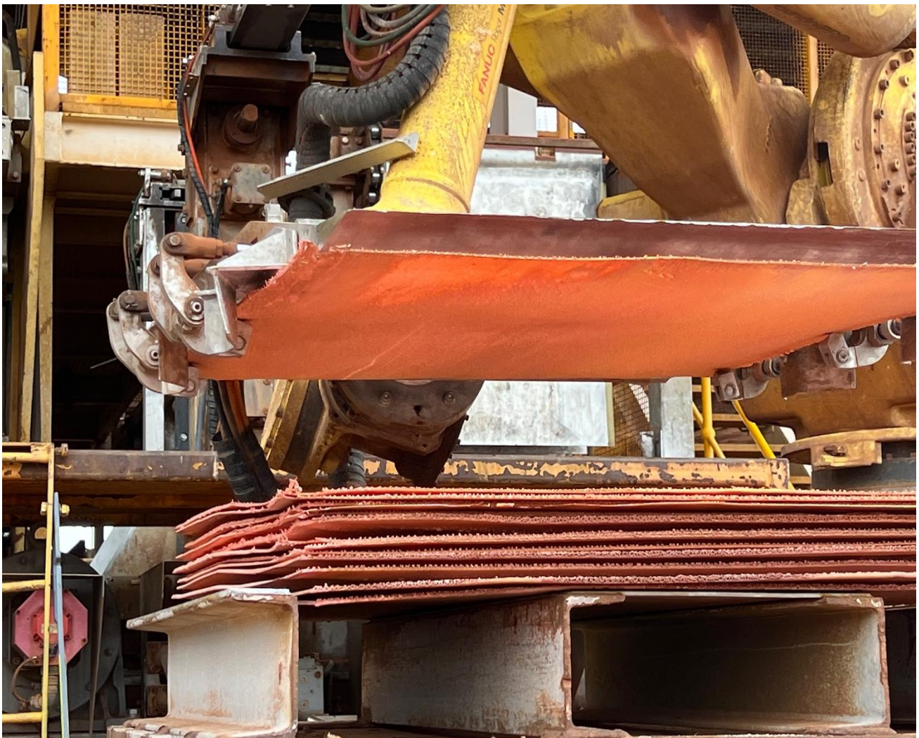
Image 1. Copper cathode sheets being robotically stacked prior to bundling and shipping to Townsville Port for sale.
