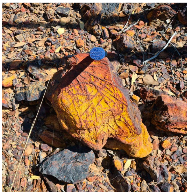
Outcropping iron rich goethite at Dividend prospect, 2km east of the Flying Horse pit. Surface sampling returned copper values between 0.1% and 0.5% Cu.
