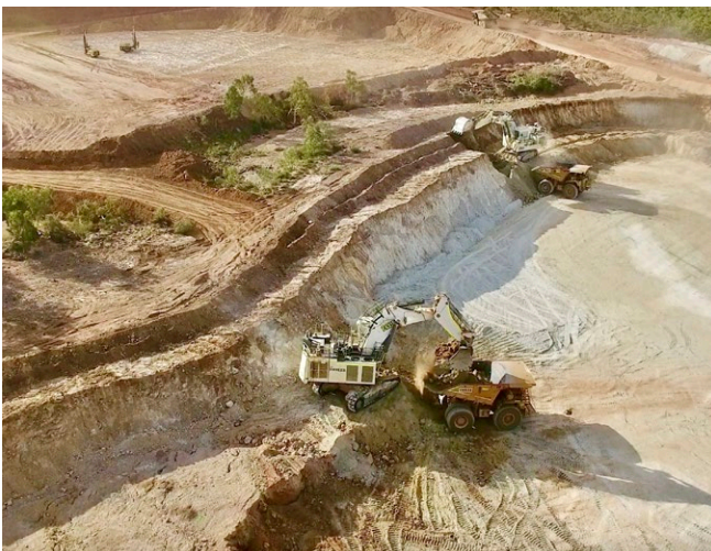
Excavators and drills working at Anthill east pit.
