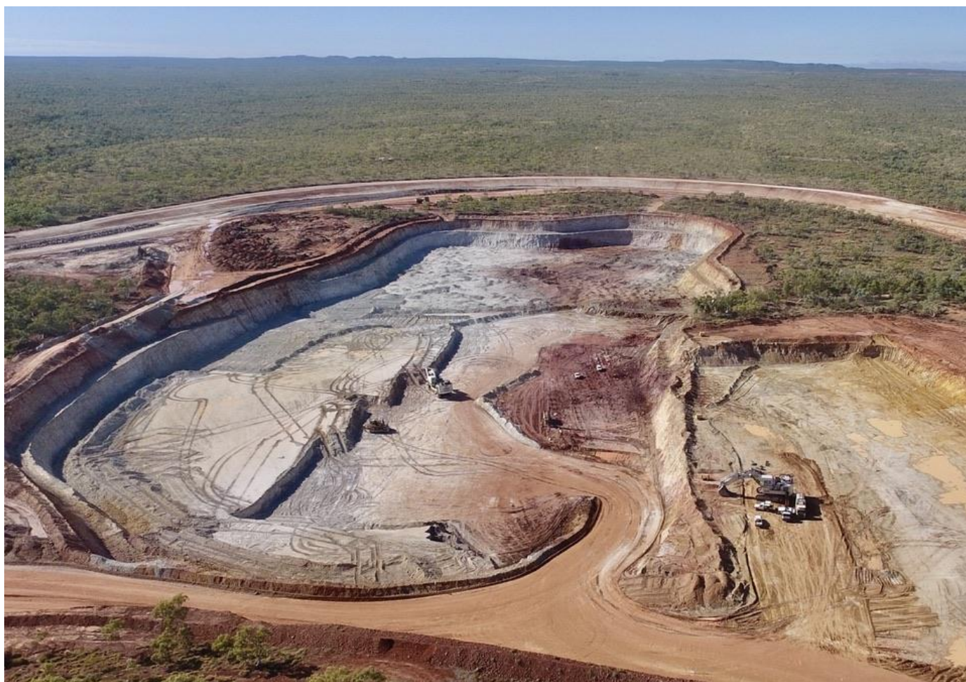
Figure 1. Anthill Mine east pit, 27 April. 5.7Mt of overburden moved between January and April 2022. Oxide copper ore appears in the right half of the main pit as dark coloured material. 100,000t of ore was mined in April 2022.
