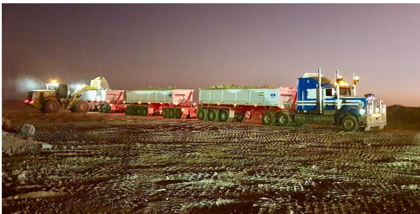
Figure 2. Road train being loaded with Anthill ore before travelling 43km to the Mt Kelly processing plant.
