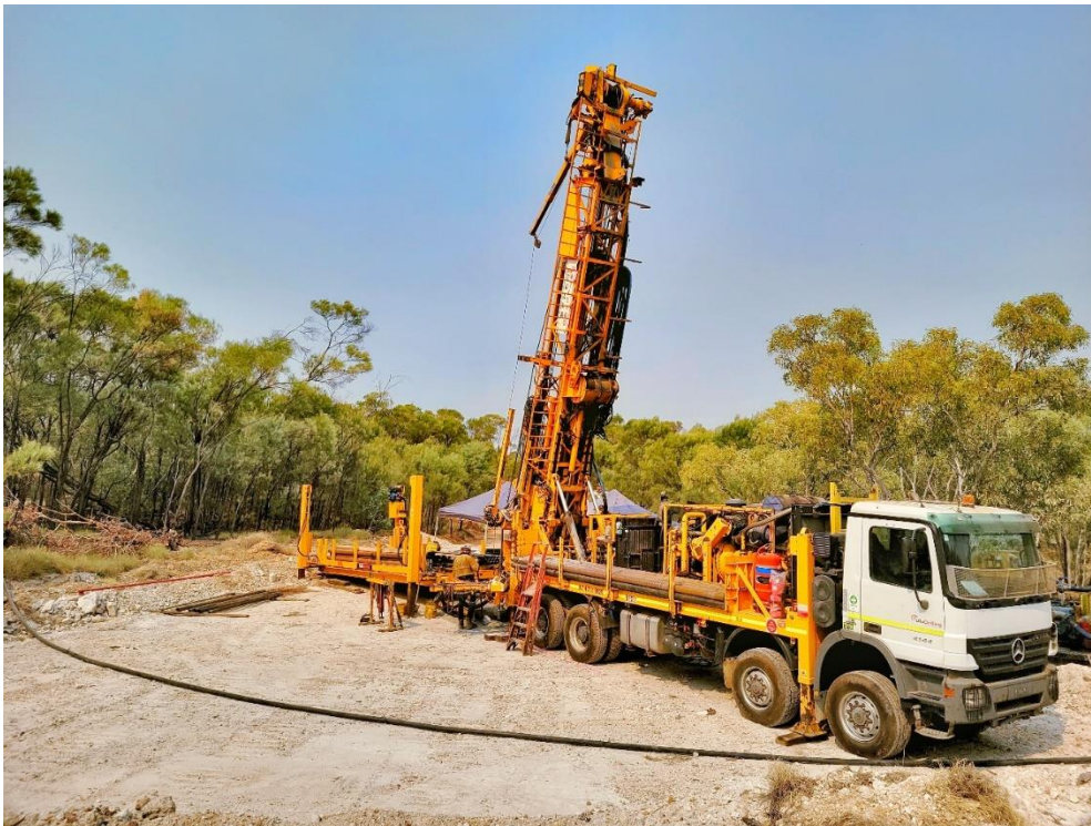
Figure 14. Tulla UDR1200 drilling at Lady Colleen prospect.
